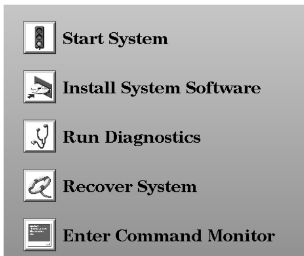
Figure 3-3 The System Maintenance Menu
